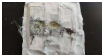
Figure 1: No perforation of all the 7.62mm AP bullets on the 3D Textile composite protection.
