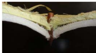
Figure 2: Perforation with 12.7mm AP ammunition through the 3D Textile composite structure.
