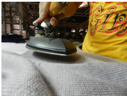
Figure 9: Iron and Knitwear surface distance Figure 10: Seam must be ironed 1 cm to back
