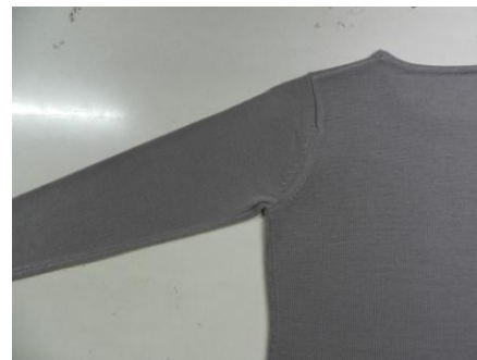
Figure 9: Iron and Knitwear surface distance Figure 10: Seam must be ironed 1 cm to back
