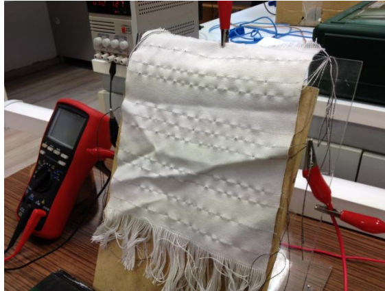
Figure 2.2 Connection of the power supply to fabric.
