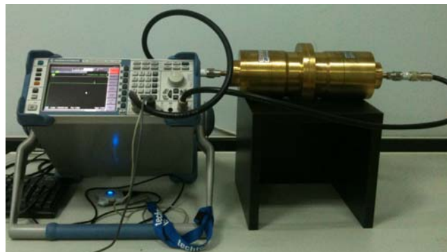
Figure 4: Set up of EMSE Testing Apparatus
