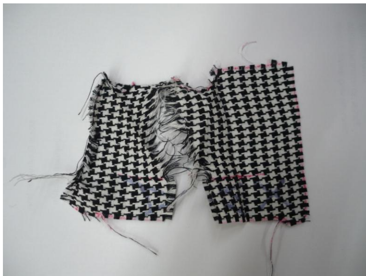
Figure 3: Puckering of specimen
