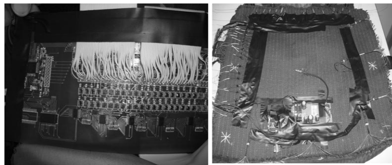
Figure 2: Flexible PCB for Bullet impact detection and 80 x 80 POF Integrated Garment
