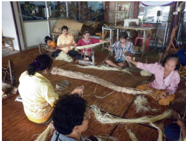
Figure 11: Twisting fiber into yarns
